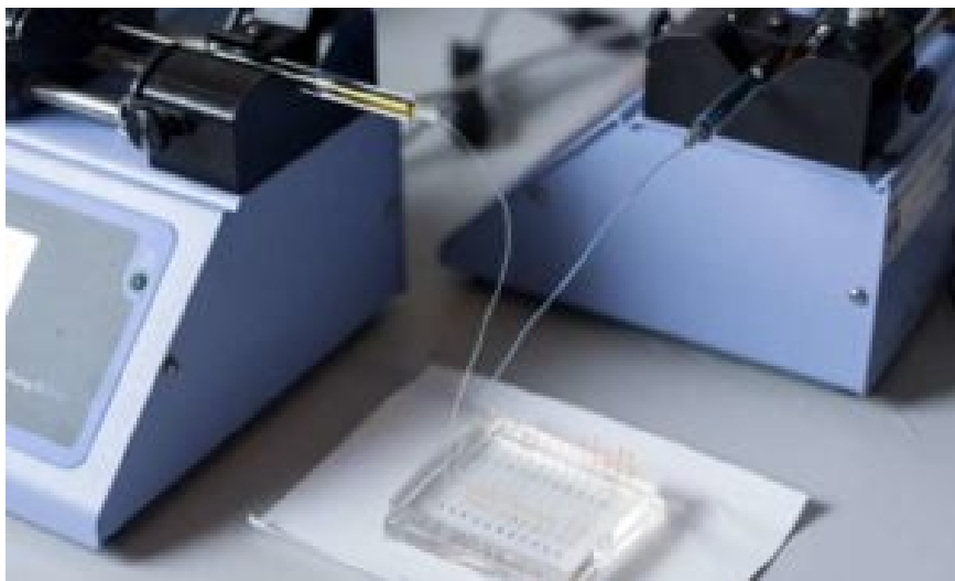
A microfluidic chip used to fabricate nanoparticles that could be used to deliver therapeutic genes to specific organs of the body. Credit: Rob Felt, Georgia Tech
