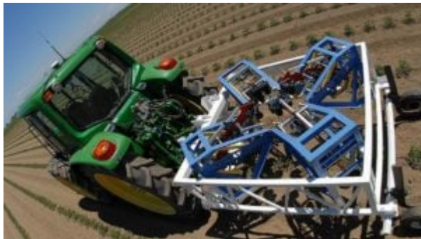
The new tractor-drawn phenotyping machine, developed at UC Davis, can measure three plants per second, using advanced sensor technology. (Photo: David Slaughter, UC-Davis)
