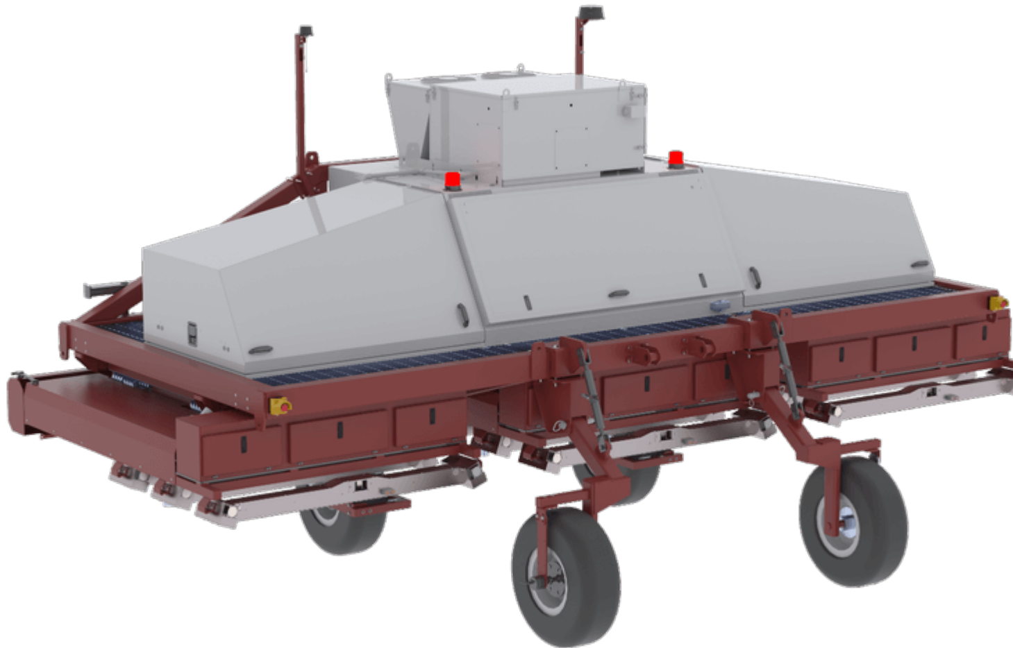
Laser wielding robot that kills weeds. Credit: Carbon Robotics
